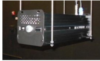
Luminaire mounted on goniophotometer
