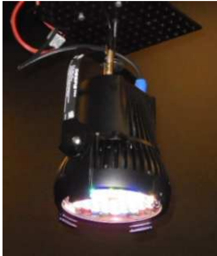
Luminaire mounted on goniophotometer.
